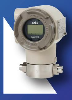
The Model CVM400 Natural Gas Calorimeter measures the thermal conductivity of a gas mixture such as natural gas at different temperatures and calculates the calorific value of the gas based on its thermal conductivity.
