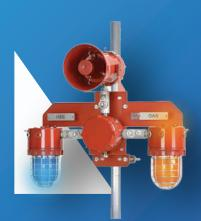
The audio-visual alarm station is designed for installation and use in heavy industrial environments. The alarm station consists of a beacon and alarm horn. The warning light comes in field interchangeable dome colors of amber, blue, clear, green, red, yellow and magenta.
